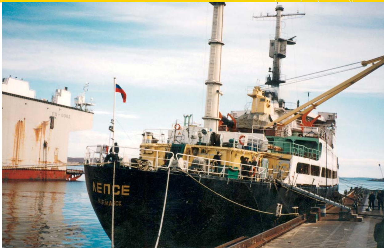
The ship "Lepse", moored at a quay near Murmansk, is used as a storage vessel for spent fuel from nuclear-powered ice-breakers. Photo: Norwegian Radiation Protection Authority
