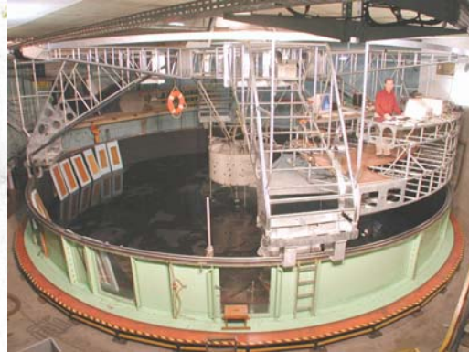
Coriolis lab in Grenoble: Rotating tank, diam = 13 m
