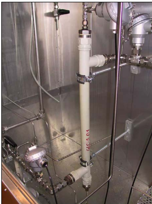
Figure 6. Laboratory membrane absorber module. (Range 25 - 70oC, < 1.5 bars CO2 pressure)
