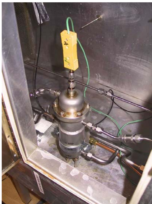
Figure 2: This apparatus can operate up to 7 bars and a temperature of 130°C
